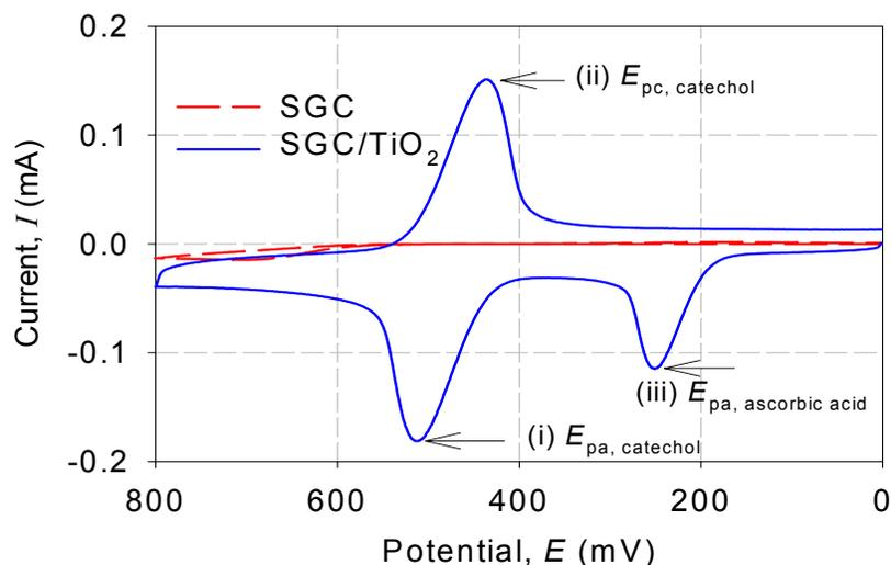
**Figure 2 (a):** Cyclic voltammogram of 5mM catechol +5mM ascorbic acid in 10 mM H<sub>2</sub>SO<sub>4</sub> (100 mV/s) vs Ag/AgCl /3 M NaCl, on bare sonogel-carbon electrode (Bare SGC, Red Line) and compare to (SGC-TiO<sub>2</sub>, Blue Line) modified electrode [current (mA) vs. potential (mV)].
