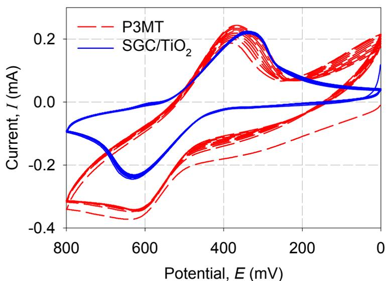
**Figure 2(b):** Comparison of the stability of SGC/TiO<sub>2</sub> electrode (Blue Line) and P3MT modified electrode (Red Line) in the detection of 5 mM catechol in 10 mM H<sub>2</sub>SO<sub>4</sub> (100 mV/S) over 20 scans [current (mA) vs. potential (mV)].
