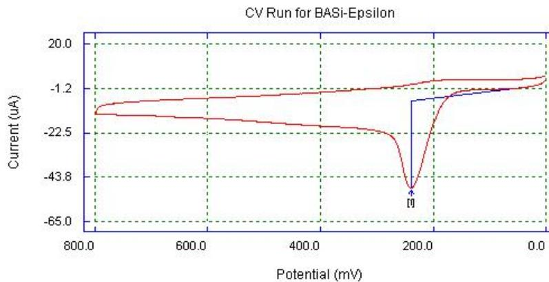
Cyclic voltammogram of 5 mM ascorbic acid in 10 mM H<sub>2</sub>SO<sub>4</sub> (100 mV) vs. Ag/AgCl/3M NaCl on SGC/TiO<sub>2</sub> modified electrode (Irreversible ascorbic acid).
