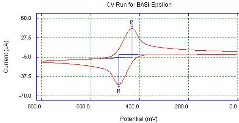
Cyclic voltammogram of 5mM catechol in 10 mM H<sub>2</sub>SO<sub>4</sub> (100 mV/s) vs. Ag/AgCl /3 M NaCl, on SGC/TiO<sub>2</sub> modified electrode (Reversible catechol).
