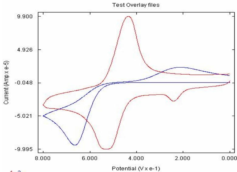
1 SGC/TiO<sub>2</sub> and 2 P3MT: cyclic voltammogram of 5 mM catechol + 5 mM ascorbic acid in 10 mM H<sub>2</sub>SO<sub>4</sub> (100 mV/s). This data allows the student to see that the SGC/TiO<sub>2</sub> can distinguish there is ascorbic acid and catechol present where with the P3MT electrode there is no peak for ascorbic acid and the peak difference (cathode –anode) is much greater for catechol detection.
