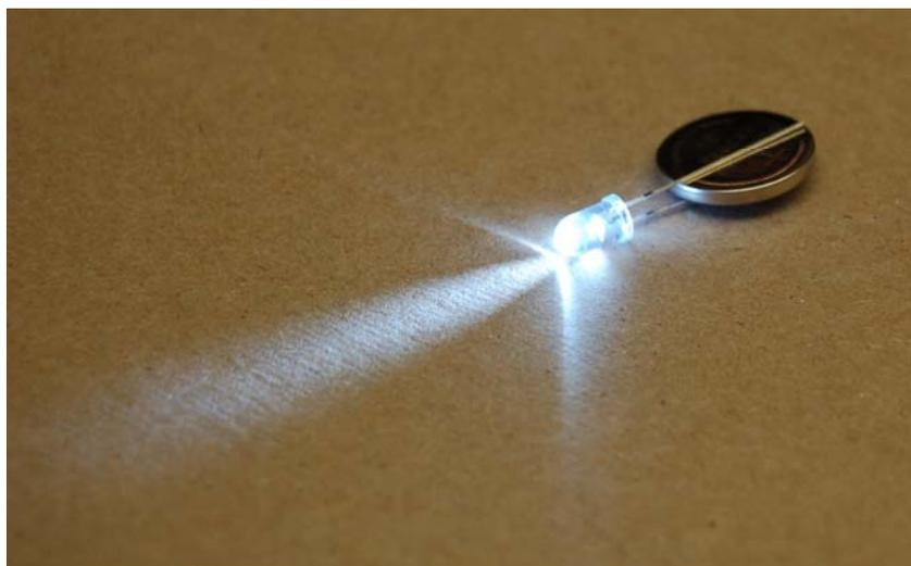
**Figure 3.** LED and Battery. LED diameter is 5 mm.
