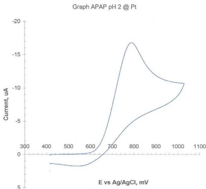
Figure 3. Cyclic Voltammogram of APAP in pH 2 buffer at a Pt electrode. Scan rate is 100 mV/s.
