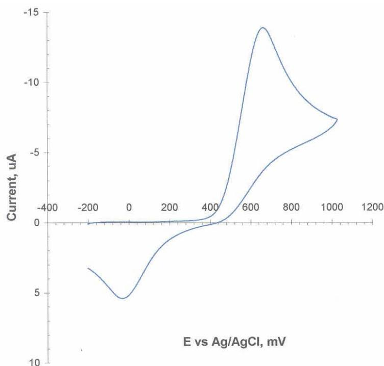
Figure 2. Cyclic Voltammogram of 2 mM APAP in pH 7.0 buffer at a glassy carbon electrode. Scan rate is 100 mV/s.
